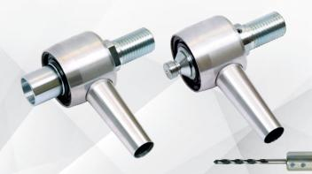
The CEBOR extraction rotor enables dry drilling with drill motors that are not prepared for dry drilling with dust extraction. For this purpose, the rotor is placed between the drill spindle and drill bit.
