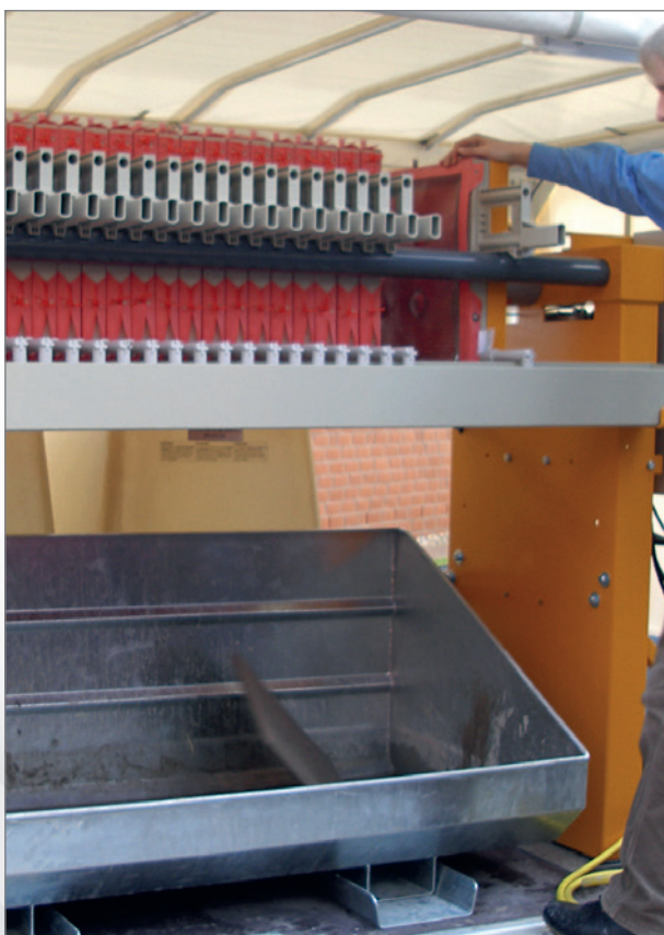
The filter is emptied by tearing apart the filter elements.
