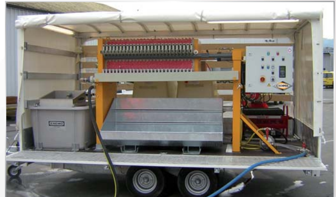
left: collecting basin with strainer; centre above: filter element; centre below: solids container
