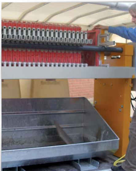
the filter is emptied by tearing apart the filter elements
