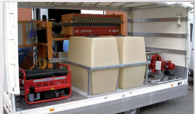
from left to right: current generator, clear water tanks, slurry pump
